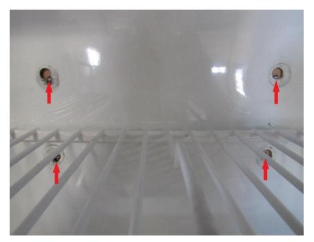
Do the same with the refrigerator fin. Install screws pulling it tight. Fin fan can now be attached to the center of the fin
