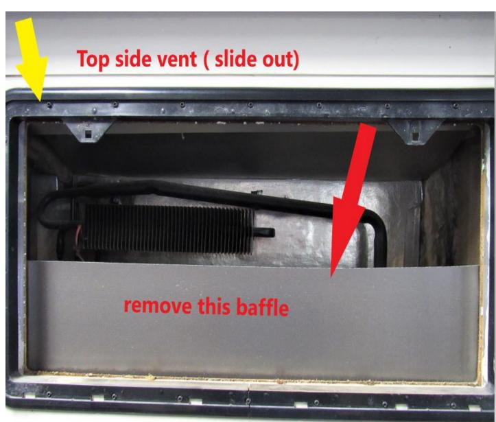
You will then be required to add a slideout fan to your top side vent to force the hot air out that's being pushed up from the fans below the vent, (this is required on all slide out models to be covered in our warranty)
