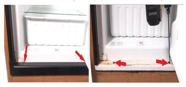
Take a 5/16" hex bit and cordless impact driver and proceed to loosen all the screws (RA) in the freezer and the refrigerator. Unclip thermistor and leave it hanging down into the fridge box. Removing your freezer shelve or top fridge shelve is optional.
