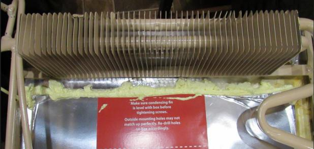
In some areas it might seem to be tight against the box, and in this area cut back enough foam on a angle to create a small gap off the unit so you can get your foam straw in to fill the void further down.
