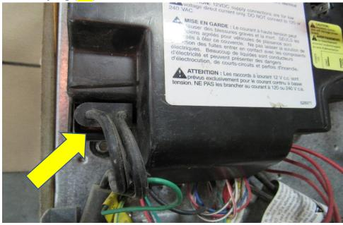
Remove the board cover and then remove the heating element wires. (RA)
