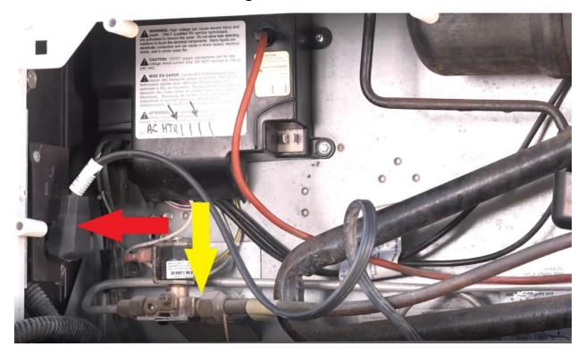
There are many different styles out there but most have at least 2 mounting screws through the back plate holding the fridge to your RV floor. Screw size and bit needed will vary from coach to coach. Remove screws or Bolts (RA).
