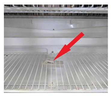
The same applies the with freezer. Clip the sensor underneath the shelf, centered from side to side, but have this one more towards the back of the freezer.
