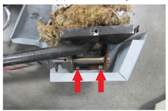
Remove the igniter and burner screws (RA). These are usually Phillips screws.
