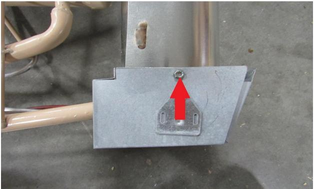
If you bought new heaters with the unit this can be disregarded as the correct heaters will be sent with the new unit. The heaters should be snug but not really tight or floppy loose. This model has 2 heater styles, 1 is a 45deg angle 3/8" and the other is a 90 deg angle 7/16" if you are keeping your old heater then this should have been clarified which style you have when you ordered.
