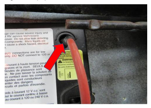
Take the 120V plug (YA) loose from the board in order to remove the cover.
