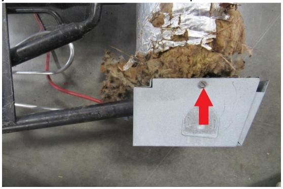
Remove the 1/4" screws (RA) and set the burner housing to the side.
