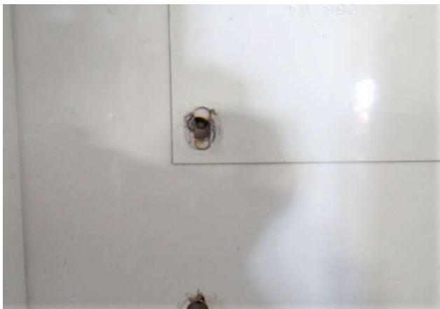
When holes are lined up, install the 7 freezer screws (RA), if you are wanting to use new screws use a 2" X #10 screw, pull the unit tight against the back. If holes do not line up exactly you can easily angle the screw up/down side/side to get to the hole as these holes are set in approx. 1" from the front surface of the foam pack.
