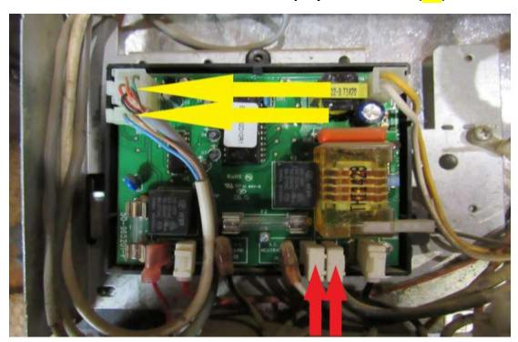
Remove the power wire (RA) and the small red/black light wire (YA).
