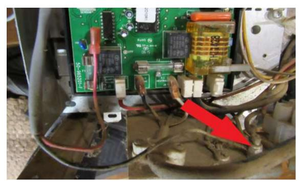
Cut the zip ties that hold the front display wire and the thermistor wire to the cooling unit and pull them out from under the coil so that they don't interfere when removing the cooling unit.
