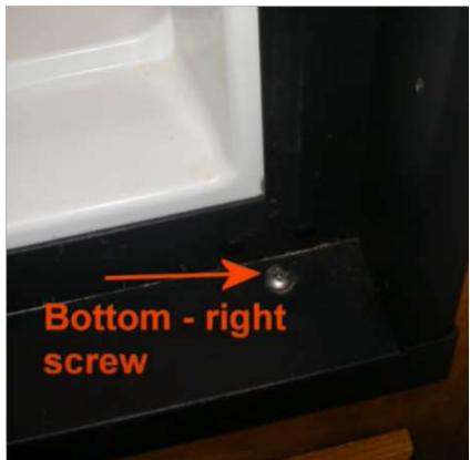
Take a Philips bit and cordless impact driver and proceed to loosen all the screws (RA) and in the freezer and on the fins in the refrigerator (Screw head & length may vary). Also unclip thermistor (YA) and set to the side.
