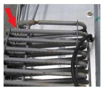
The fridge fins will sometimes separate from the cooling unit when you pull it off but they also sometimes remain attached to the cooling unit, as seen in the picture below.
