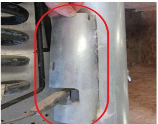
Clean off all the old thermal mastic and remove any tape (RA).
