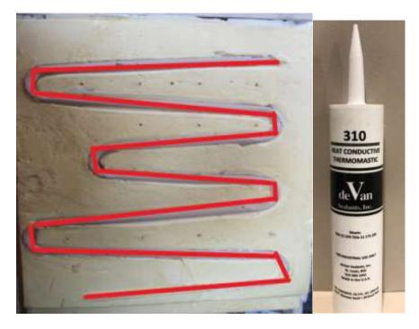
Lay cooling unit into box, being careful not to scrape off thermal mastic. There are many different models, so your exterior mounting screws might not line up perfectly which is normal. Install 1 mounting screw on the bottom and 1 on top.
