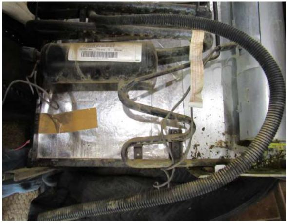
Remove the old cooling unit from the box. Start by lifting the bottom of the cooling unit. If it doesn't want to lift out, you can use a pry bar and get it between the coils and the fridge (RA) box and pry up. This should get it started. Then continue to pull on the cooling unit until it is completely out of the cavity.
