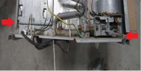
The drain hose is sometimes routed through the coil. If this is the case, pull it out so that it doesn't get caught when removing the cooling unit.
