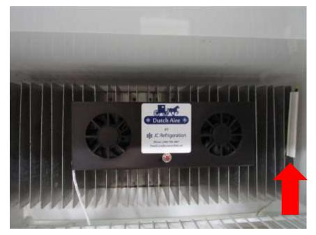
The thermistor should be located on the 1<sup>st</sup> fin from the right side. (See above picture, red arrow)
