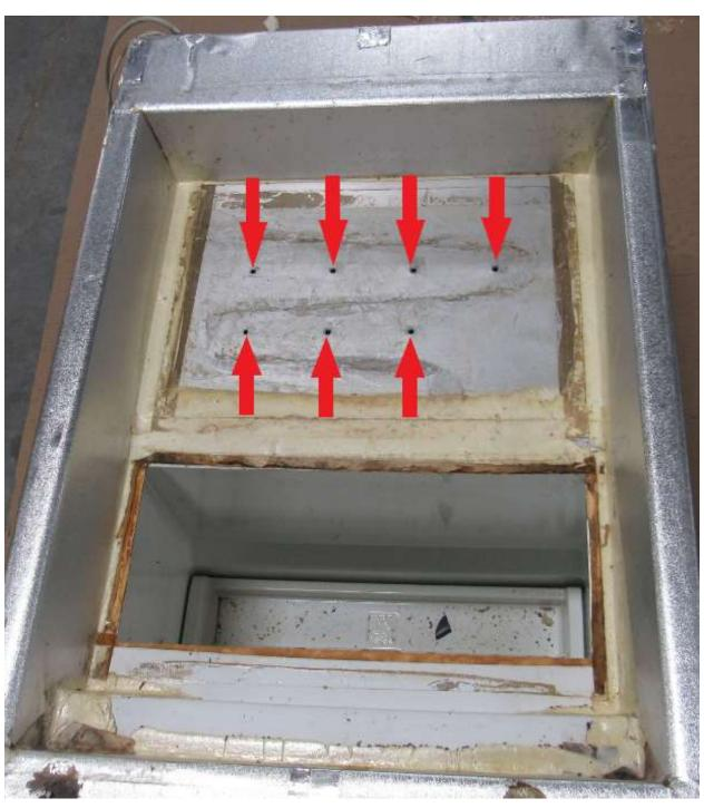
If you bought a new heating element, insert it into the new unit as shown. Push the insulation back so the heating element sockets are exposed, and slide the heating element into the socket. It does not matter which socket you chose. Make sure it's pushed all the way down to the stop point on the heating element. Push insulation back over the heaters and install the cover we took off of the old unit and tuck the heater wires out of the way for now.
