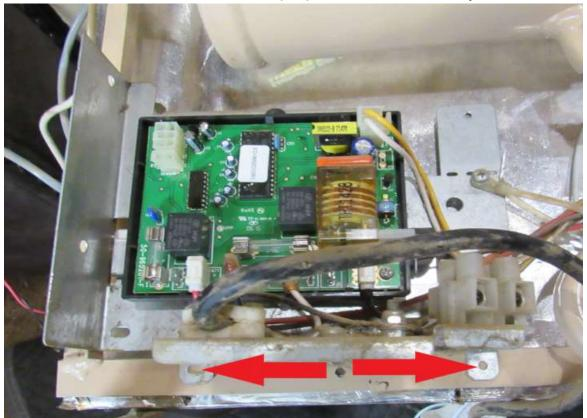
Loosen these screws (RA). We will tighten them in the next steps. On some models this burner bracket will not be used
