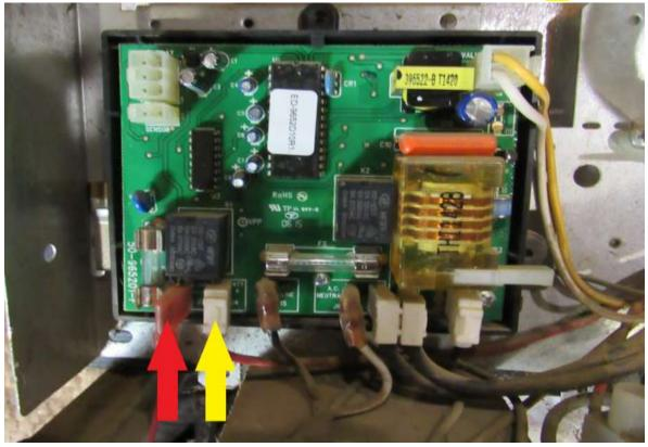
The black wire needs to be removed from the ground terminal (RA). It will need to be put back at the same location later. We normally just cut it then splice it back together later
