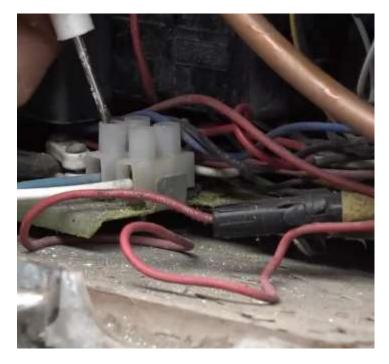
The wires ends are not insulated so use a piece of tape or a twist cap to protect the end of the 12V + wire. This will keep it from accidently touching a ground and blowing a fuse. It will also let you know which one is the 12V + wire once you go to hook everything back up at the end.
