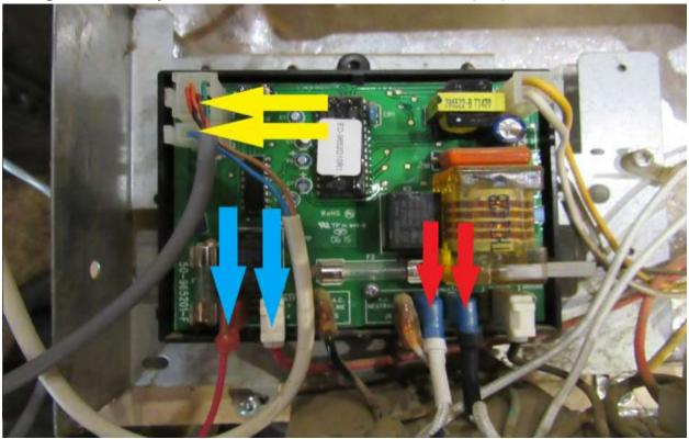
Reconnect the black ground wire to the terminal (RA). Or if cut splice together again
