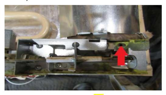
Re-install the gas valve holder screws (YA) retighten screws (RA).
