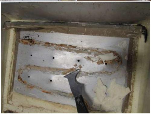
If the original cooling unit pulled the freezer plate inward at the holes for the screws, you want to flatten the area around the hole or you won't have a good connection between the freezer plate of the new cooling unit and the fridge box. These can be tapped down using a hammer. <a href="NOTE:">NOTE:</a> If the fin was removed make sure to put this back in right side up as it was, otherwise your holes will not line up once the new unit gets installed.
