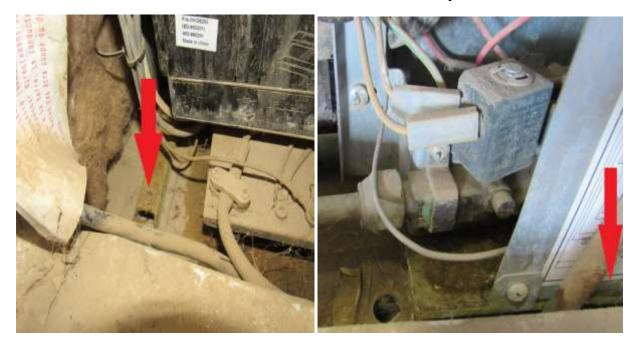
Now you will go to the inside of the coach to remove the mounting screws from the front of the fridge. To remove the top cover, use a flat screw driver and insert it into the slot to release the cover. (Styles may vary)
