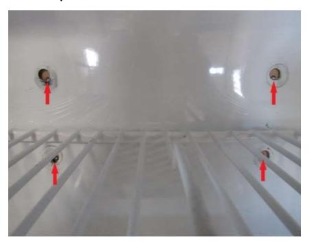
Do the same with the refrigerator fin. Install screws pulling it Evaporator fin up tight.
