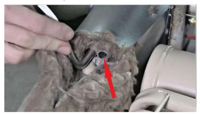
Lay the unit on its back and place a small bead of thermal mastic as shown in red. You will need to use the the entire tube.
