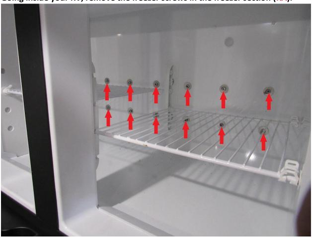
Remove the screws from the fin in the refrigerator (RA). Also remove the clear defrost tray and set aside (YA).
