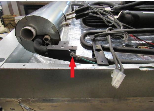
Lift the unit straight up and out. Have someone pull the thermistor wire down through the hole in the unit as the unit is lifted out (RA). Thermistor should not be removed from box, but left clipped to the inside of the fridge. If you have a ice maker then the icemaker water spigot/heater wire needs to be pulled thru the unit on top as well when you lift up.
