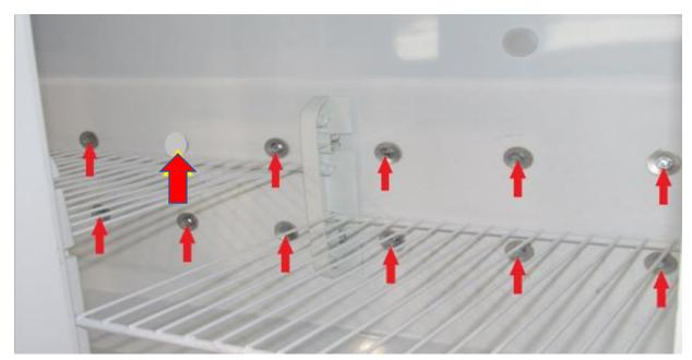
Install all the screws into the refrigerator fin (RA).
