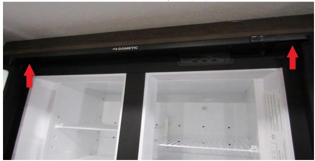
Fasten the two mounting screws back into place (RA).
