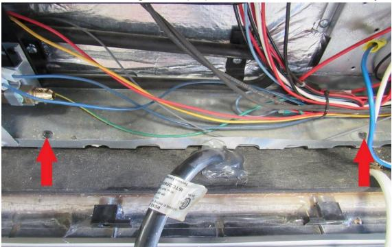
Make sure your water line is turned off (BA), remove the water supply line for the icemaker/water dispenser (GA). If your defrost hose is connected to a drain hose disconnect it from the coach line, most times this hose is loose in the back and so no need to loose from coach (RA)
