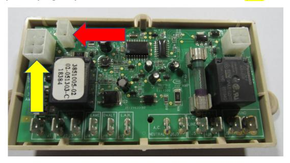
This is the more common board: Take a screwdriver and gently pry out both sides of the board to release the cover (RA).
