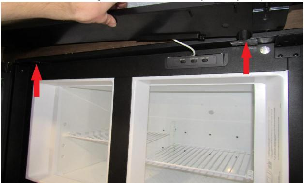
Fasten the top control panel back into place with the same screws you just took out so it doesn't get damaged (RA).
