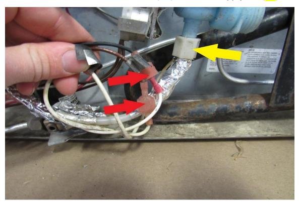
Disconnect the 120V ice maker wires, mark these to make sure you know which ones they are later, because these can be confused with the 12V fan wires (RA).
