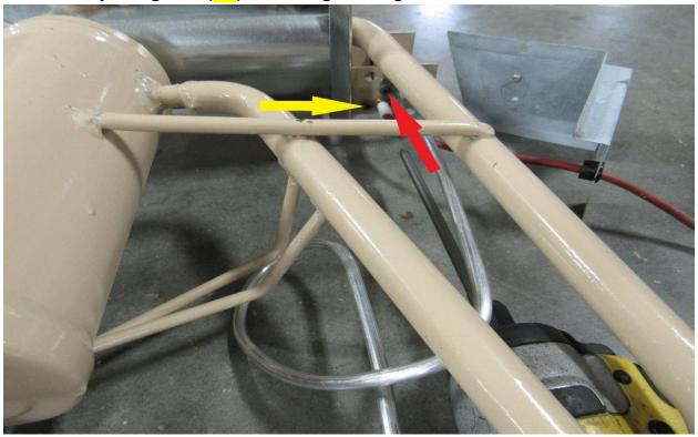
Using the original ¼" screws. Install the burner housing as shown (RA). Make sure you have approx. ¼" gap between burner tube and igniter electrode. (YA)
