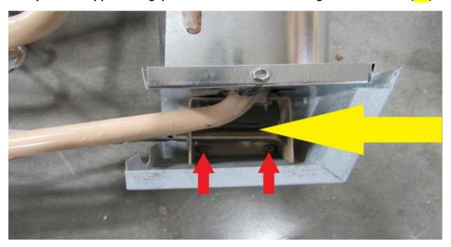
Remove the top screw from the new unit as shown (RA). We will use this screw to mount the top piece in the next step.
