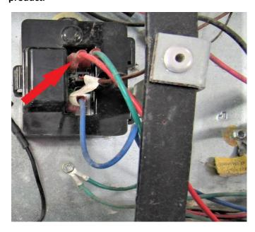
If the recall device is to be taken out, remove the blue wire (YA). Loop red wire as shown creating a "jumper" (RA). The 2 spades "limit in & limit out" should be looped together as seen (RA)
