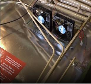
The red wire coming from the fan switch has a 3-way split. Plug the red fan wires into that as shown (RA).
