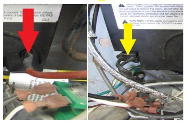
Remove ¼" Hex mounting screws on board (RA).
