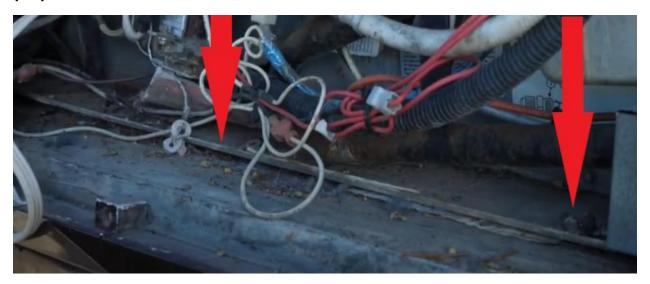
On Winnabago coachs you will have 4- 9/16" bolts lagged to a steel side plate, 2 on each side of the fridge, also the top roof vent cap needs to be removed and 2 to 4 philips screws need to be loosend from the top of the fridge.
