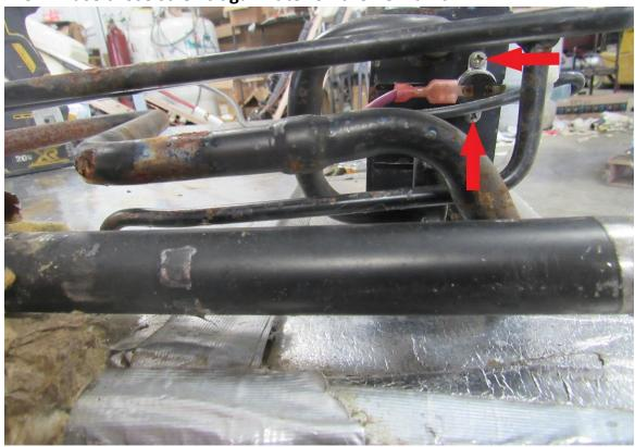
Remove the 4 fan bracket screws (RA).
