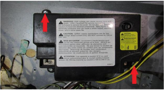
Install the three screws into the LP solenoid valve as shown.
