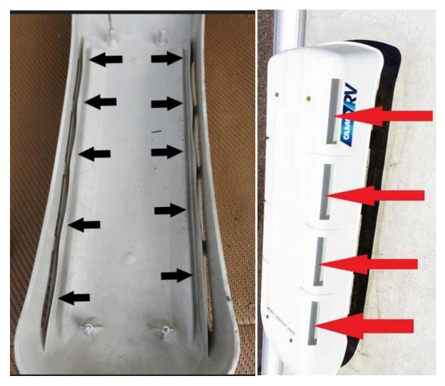
Now you're ready to slide the refrigerator back into the cavity. Once it's started it helps to have someone outside to watch as you slowly push the fridge back into place, making sure the gas line is out of the way. Attach black trim pieces on top and bottom. Install mounting screws (RA)on the top and bottom.
