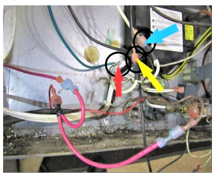
The white/or black power cord has a pigtail coming off of it and that plugs into the ice maker solenoid (RA), along with the brown wire (YA) as shown.
