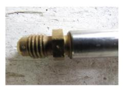
You start by taking 2 crescent wrenches and loosening the flare nut by the brass orifice, you will notice the orifice is backed away from the burner tube (above), this adjustment is done here and should stay that way, otherwise the burner will not work correctly. Do not over tighten the burner to the gas line as this might create a flare crack, yet you do want it tight enough so you do not have a gas leak.
