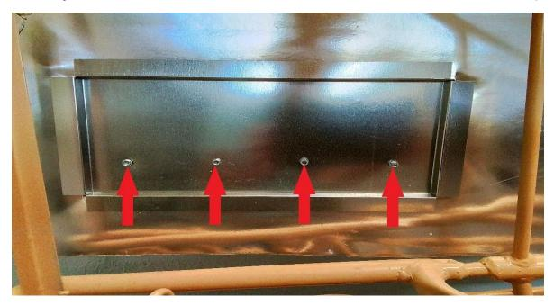
Place the fans facing up and install them using the provided screws (RA). Make sure the sticker of the fans are turned up, use only the holes that were there from the screws taken out do not make new mounting holes into this fan plate.
