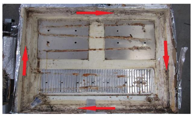
Clean off the old thermal mastic (RA) from the freezer plates and refrigerator fin. A large blade putty knife or scraper works well. A shop vac works well to remove any other debris or loose foam. Do not remove the fin as its very easy to get this back in upside down
