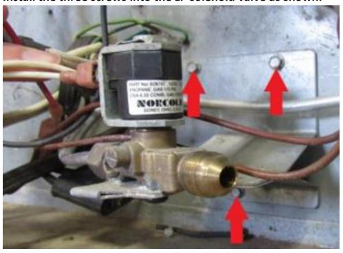
Plug the 2 gas valve wires back into the gas valve (RA)
