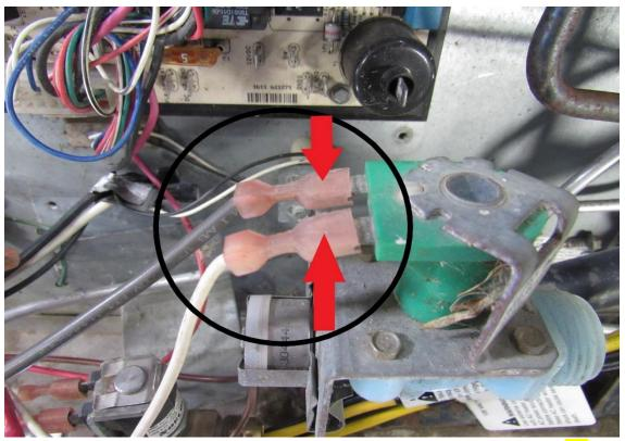
Disconnect the ice maker heater wires (RA) and water supply line (YA).
