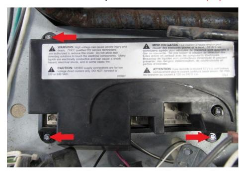
Install the three screws into the LP solenoid valve as shown.
