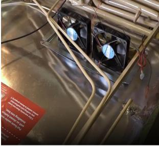
The black wire coming from the fan switch has a 3-way split. Plug the red fan wires into that as shown (YA). The white wire is the power wire coming from the board to the fan switch. (RA)
