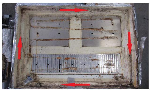
Clean off the old thermal mastic (RA) from the freezer plates and refrigerator fin. A large blade putty knife or scraper works well. A shop vac works well to remove any other debris or loose foam.
