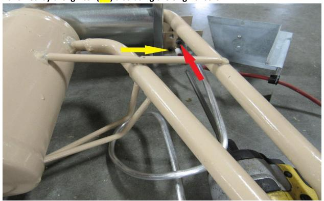
Using the original  $\frac{1}{2}$ " screws. Install the burner housing as shown (RA).
