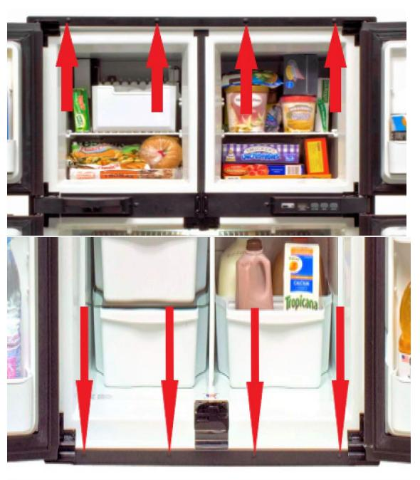
Take a 5/16" hex bit and cordless impact driver and proceed to remove all the screws (RA) in the freezer and the refrigerator.
