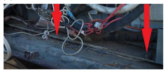
Only Winnabago coaches you will have 4- 9/16" bolts lagged to a steel side plate, 2 on each side, also the top roof vent cover needs to be removed to check philips screws need to be removed top of the fridge.
