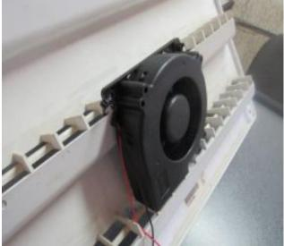
The eyelet can be screwed at any ground, connect female + to the fan switch wire, so it comes on when the lower fans come on
