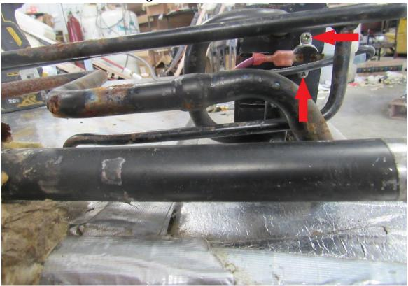
Remove the 4 fan bracket screws (RA).
