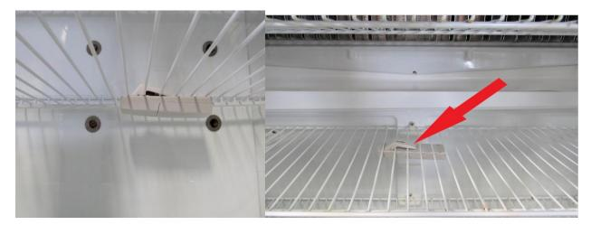
The same applies to the freezer, clip the sensor underneath the shelf, centered from side to side, but have this one more towards the back of the freezer.
